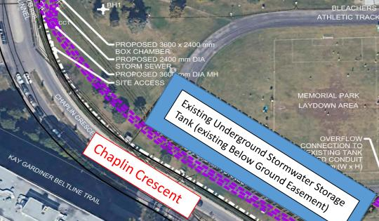
Proposed Underground Stormwater Storage Tank
